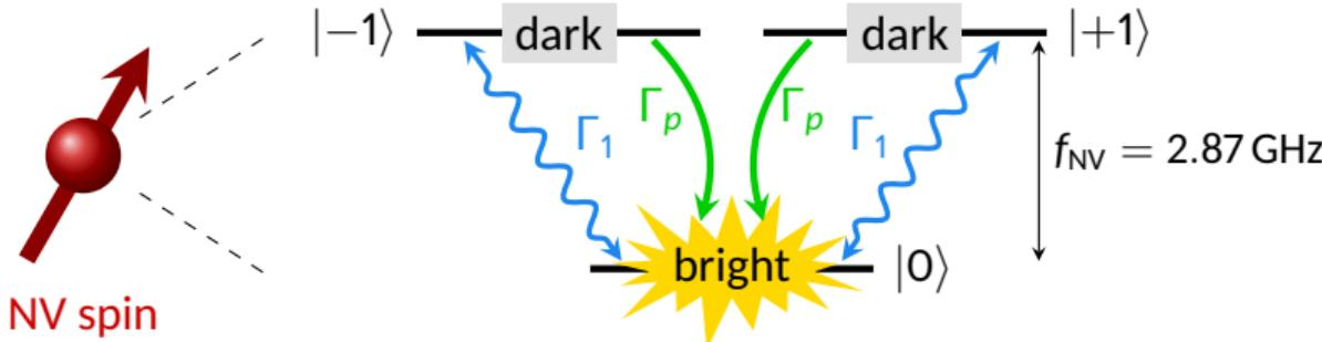
Relaxation rate  $\Gamma_1 \propto S_{B_\perp}(f_{\text{NV}})$  magnetic field spectral density at the resonance frequency  $f_{\text{NV}}$
