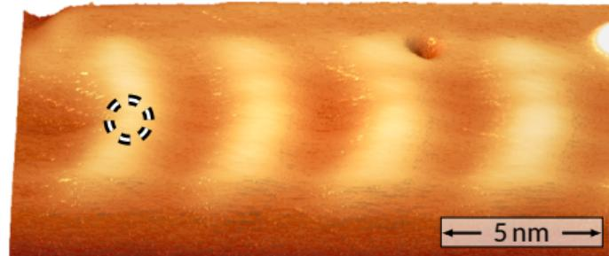
Imaging: 300 mV, 0.5 nA, 8 K, 2.5 T, Cr bulk tip
